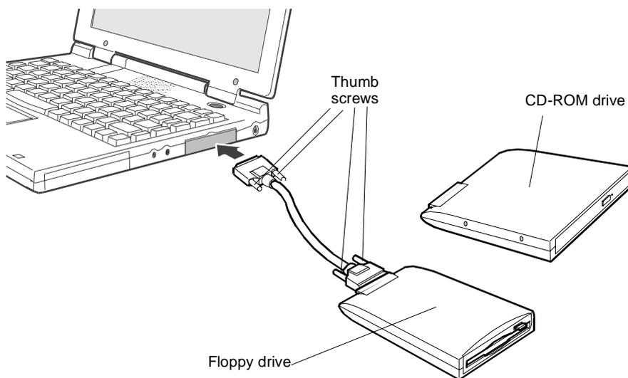
*Figure 14. Attaching the External Modules to the Computer*
