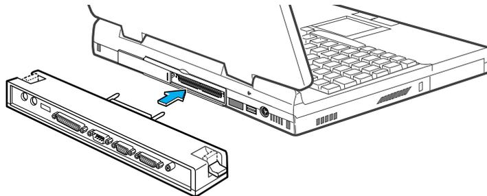
4. Move the latches on the Port Replicator into the up position.
