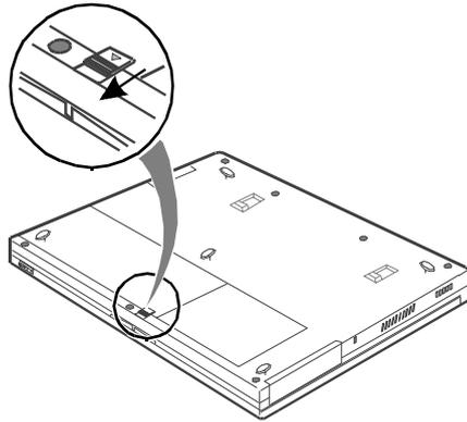
*Figure 18. Sliding the Battery Release Latch*
